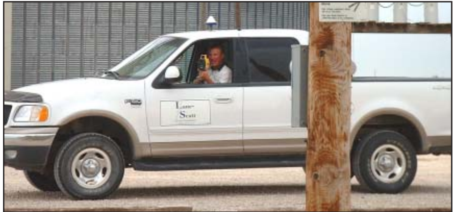
Nathan Burns Journeyman Lineman for Lane-Scott Electric Cooperative, Inc. and GPS specialist is shown here using the Lazer Range Finder from the pickup to get the GPS coordinates for this location.
