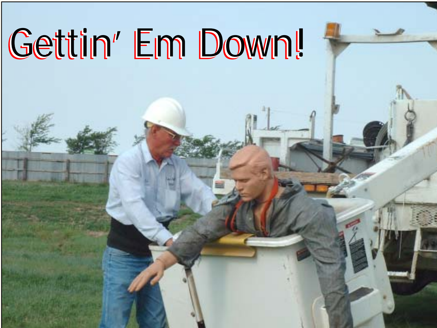
Vic Torson, Lane-Scott lineman, demonstrates the skills needed to manipulate the lift-truck's bucket to retrieve an unconscious lineman.
